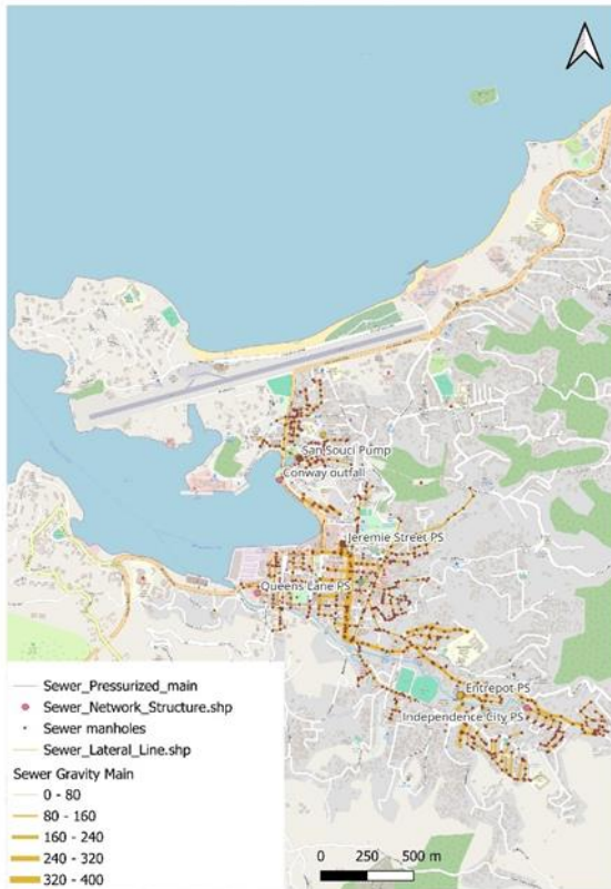
Figure 8. Layout of the Sewer System of Castries Operated by WASCO (note: there is no sewer system in Anse la Raye).
