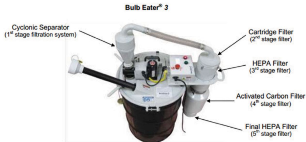
Figure 52: Bulb-Eater Device Which is Used for Mechanical Crushing of Mercury Containing Bulbs (Source: Terra Cycle)
